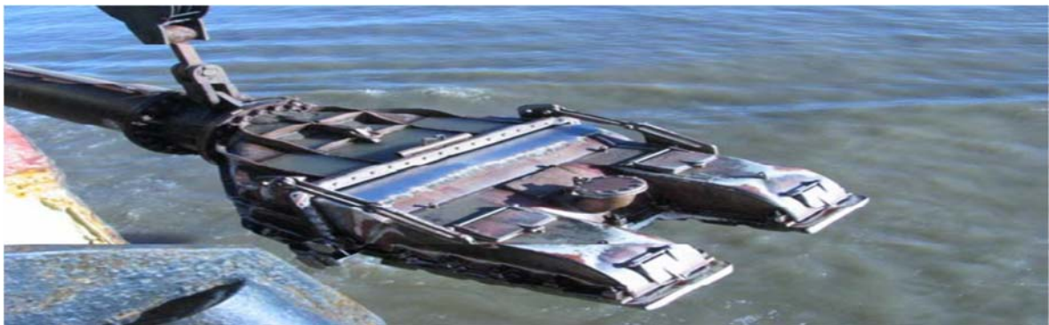
Dredging is accomplished by a drag arm on each side of the ship with a drag head at each end. As the ship navigates the channel with its dredging pumps engaged, the drag heads are lowered to the channel bottom. Like vacuum cleaners, they pull the dredged material into the ship's hoppers.
